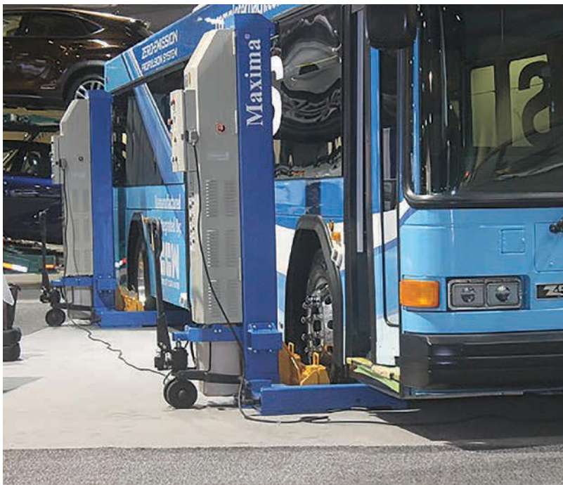
Once the lift is at the appropriate level, lock it. Make sure that it is properly locked and begin to work on the vehicle.
